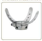
Above knee sockets require the strength provided in this lightweight, 3-prong unit. This female pyramid receiver supplies three hundred and sixty degrees of rotation, controlled by a cinch bolt.
